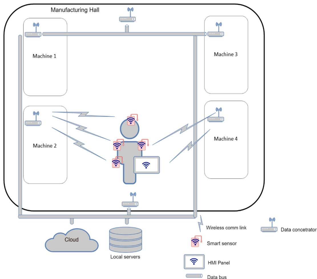
**Figure 6.** Use case I: wireless connection of the sensors at the shop floor level.
