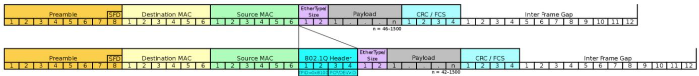
Fig. 5. 802.1Q tag in an Ethernet frame (Wikipedia, 2018).
