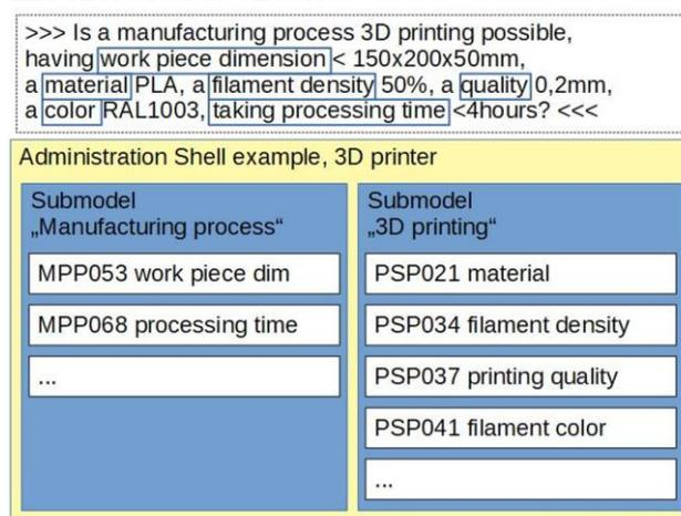
**Figure 2.** Bidding process directed towards the specific submodels of the AAS.
