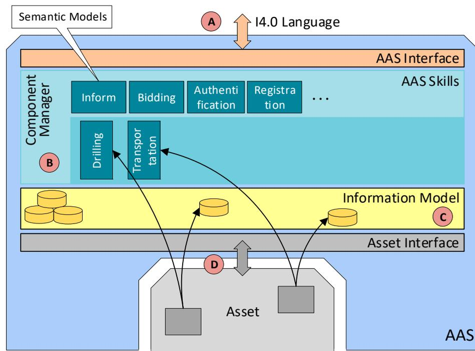
**Figure 10.** A block diagram of an AAS.
