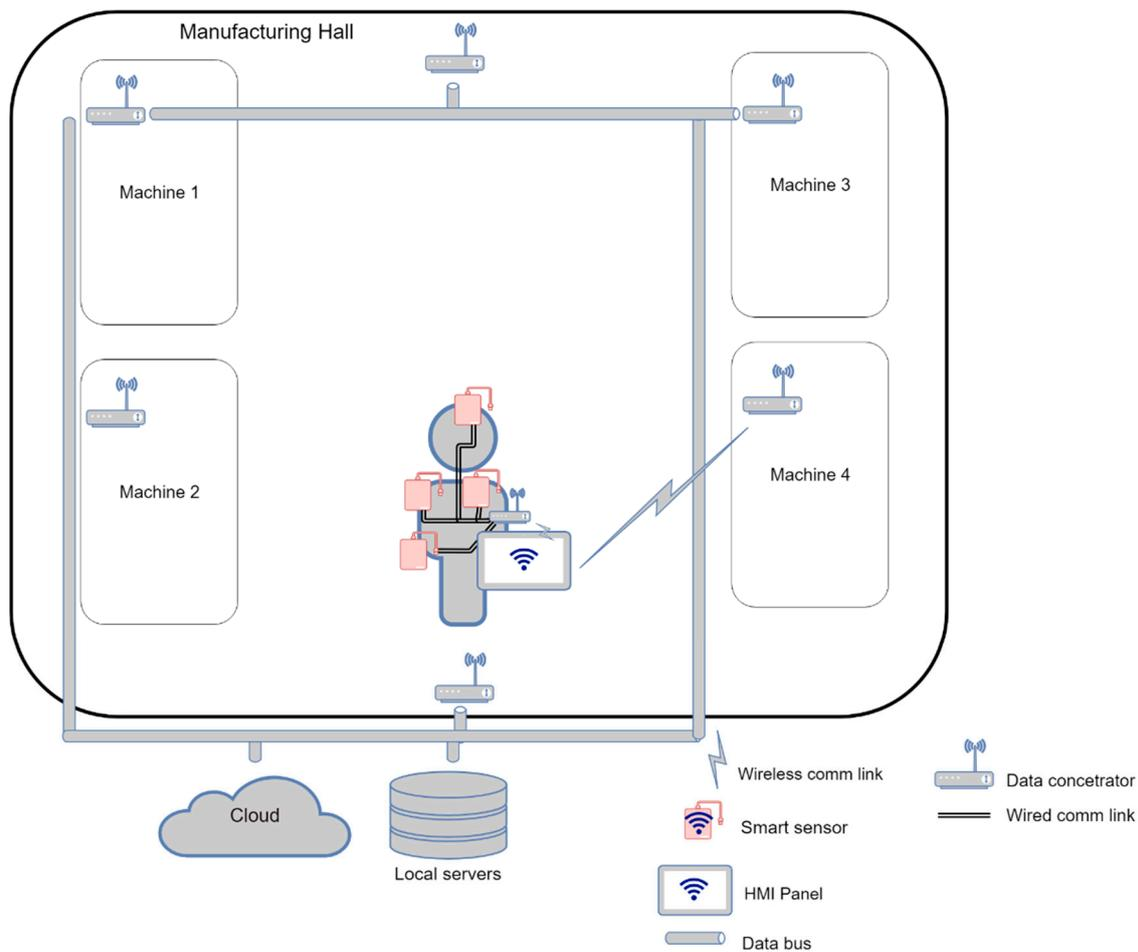
**Figure 8.** Use case III: Wired interconnection in the SmartJacket.
