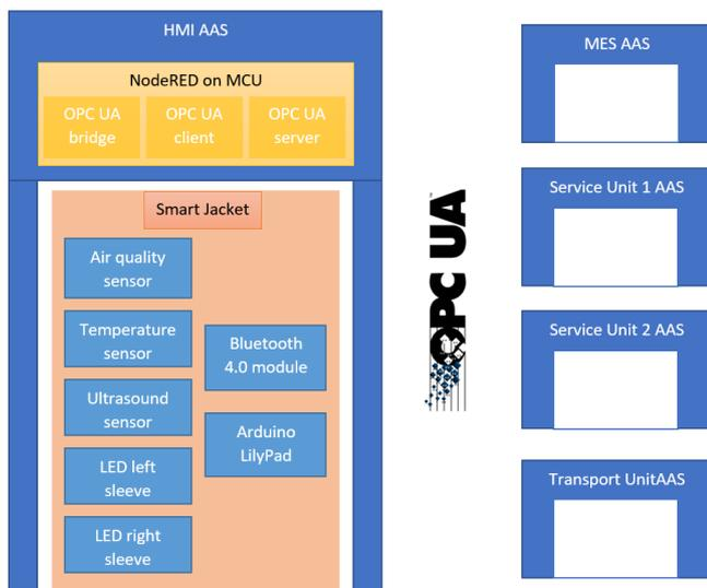
Fig. 7. A smart jacket operator represented via an HMI.
