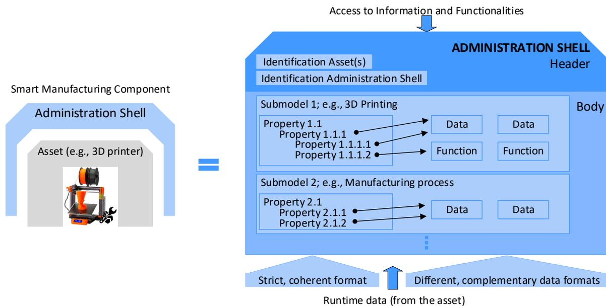
**Figure 1.** The detailed structure of an AAS.
