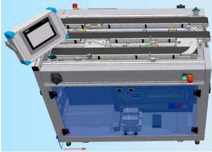
Figure 2. Basic module of a belt conveyor with a switch (Festo Didactic, 2020).
