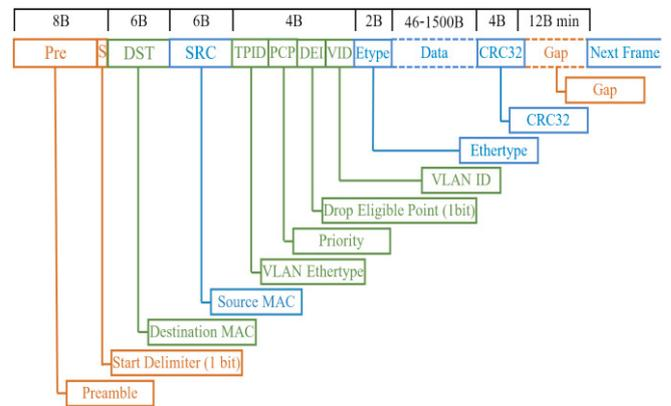
Fig. 6. An Ethernet frame with relevant parts to TSN data stream (Goller, 2019).
