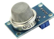
Fig. 9. An MQ-135 air quality sensor.
