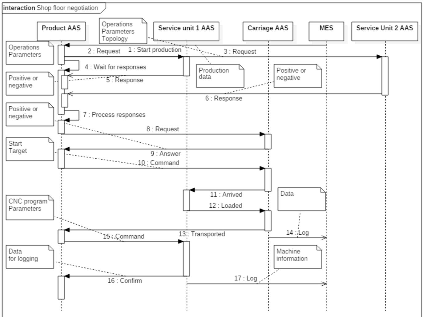
Fig. 6. Shop floor communication sequence diagram
