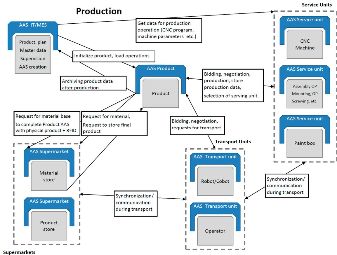
Figure 8. The data flow in a smart factory.
