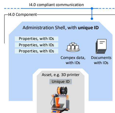
Submodels represent different aspects of an asset. Possible aspects and therefore a possible submodel could be Identification, Communication, Engineering, Configuration,
