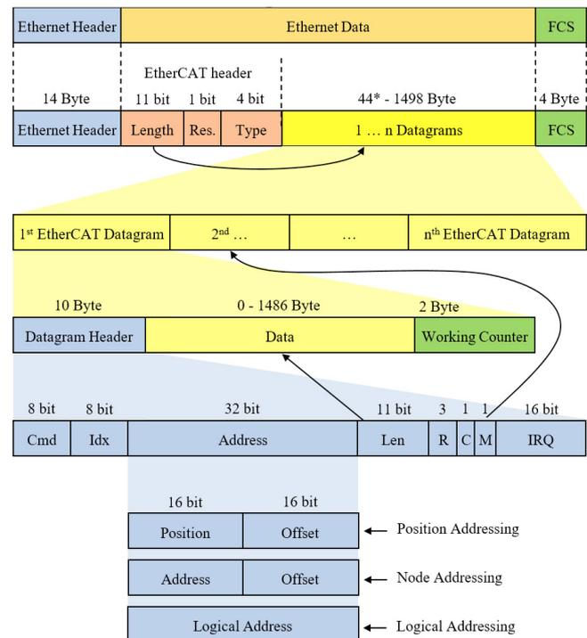
\* add 1-32 padding Bytes if Ethernet frame is shorter than 64 Bytes (Ethernet Header+Ethernet Data+FCS)
