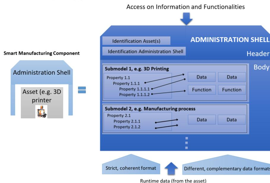
**Figure 1.** AAS Structure in details (inspired by [4,8]).
