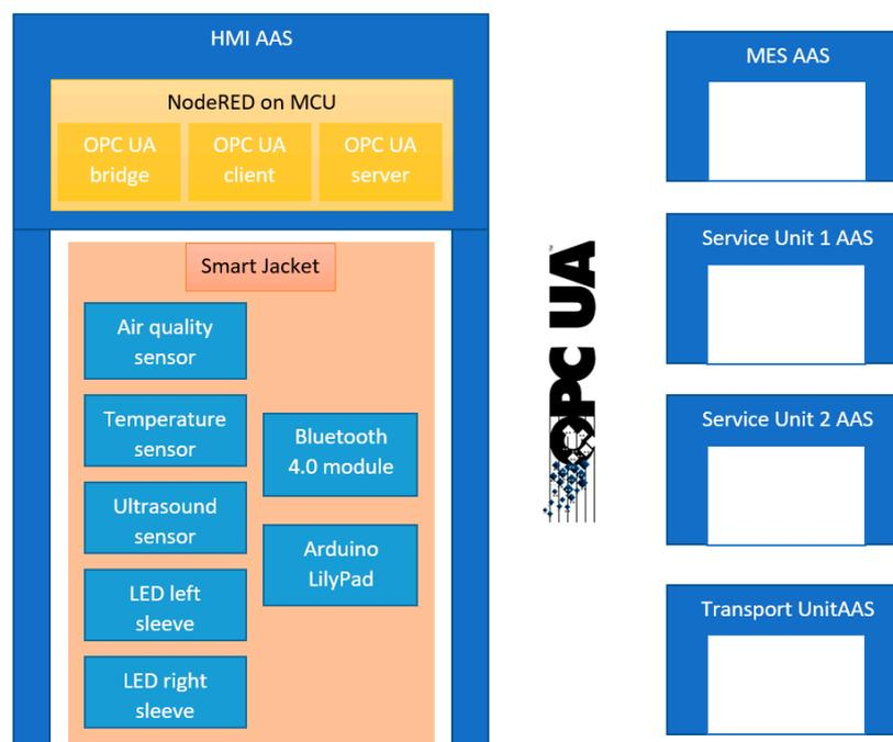
**Figure 9.** A SmartJacket operator represented via the HMI.
