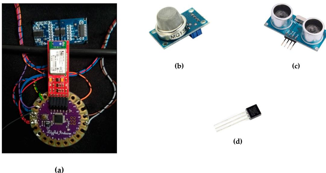
**Figure 10.** (a) An Arduino LilyPad and the wire connection of the sensors; (b) An MQ-135 air quality sensor; (c) An HC-SR-04 ultrasonic sensor; (d) a DS18B20 1-wire temperature sensor.
