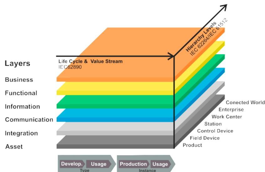
**Figure 1.** The RAMI 4.0 metamodel (inspired by ZVEI and VDI/VDE [17]).
