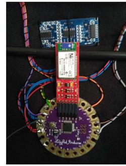
Fig. 8. An Arduino LilyPad with a bluetooth and an ultrasonic modules.
