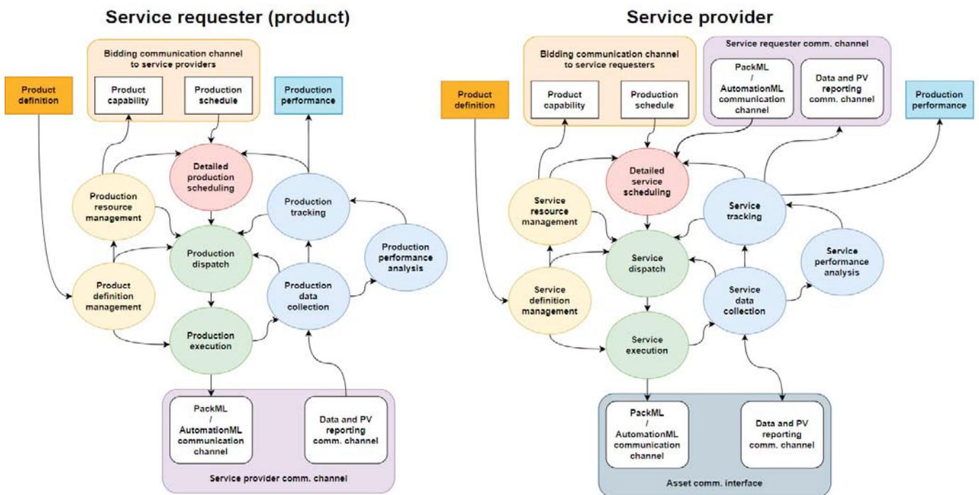
Fig. 3. Extended MOM models for Service Requester (left) and Service Provider (right)
