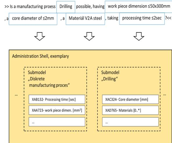
Fig. 5. An interaction pattern directed towards the domain-specific submodels in the AAS, inspired by ZVEI [5].
