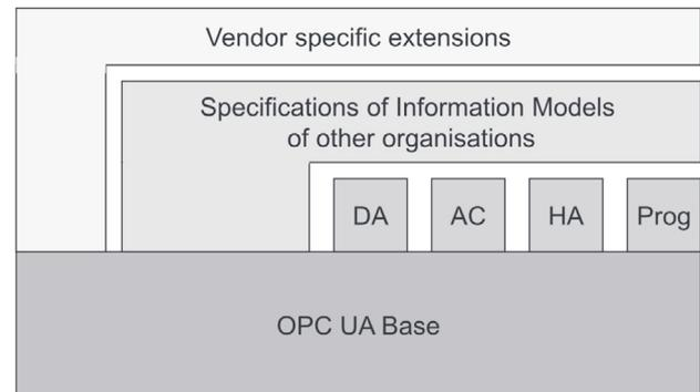
Fig. 2. OPC UA specification [Bangemann et al. (2016)]
