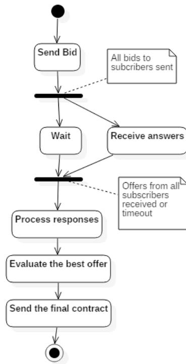
Fig. 7. The approached bidding state automaton
