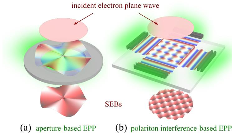
**Figure 6.1: Light-based electron phase plates.** Two possible schemes for shaping the electron wave function with light. (a) Interaction of electrons with optical field confined at edges of an aperture. (b) Electron beam shaping via the interaction with interfering polaritons.
