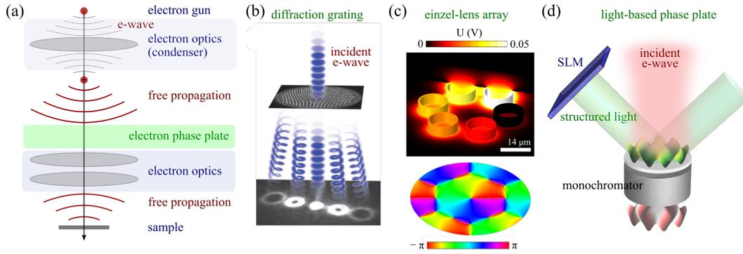
**Figure 4.1: Electron phase plates.** (a) A simplified scheme of an electron microscope with an electron phase plate. (b) Diffraction grating for generation of electron vortex beams (taken from Ref.<sup>64</sup>). (c) An array of six einzel lenses representing a tunable EPP. (d) PINEM-based EPP.
