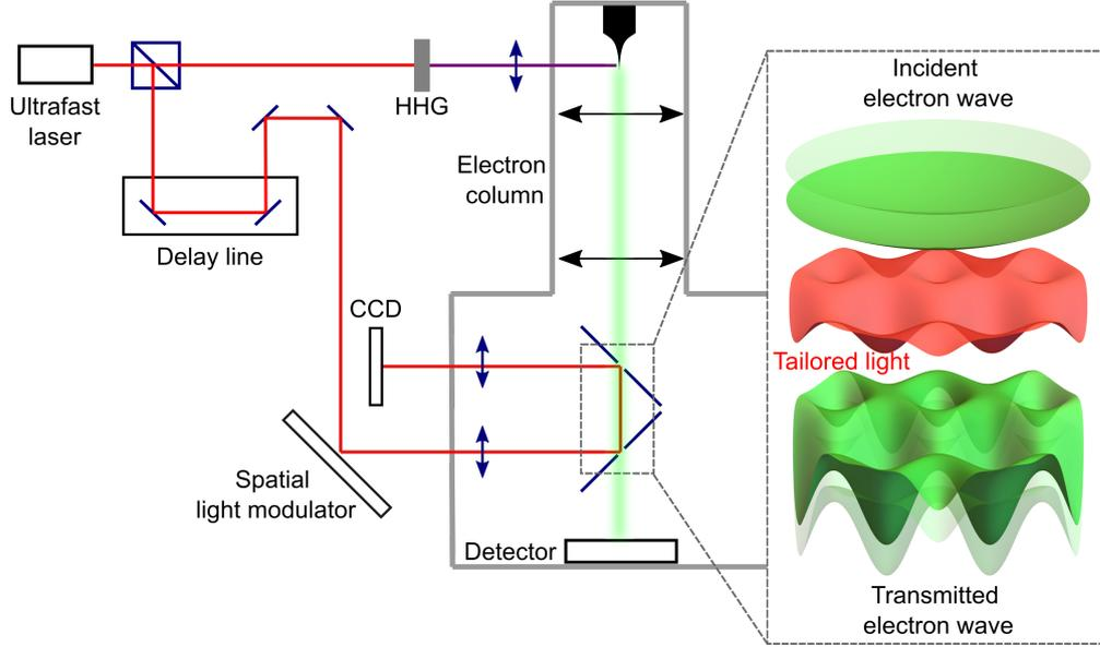
**Figure 1.2: Implementation of electron-light interaction in an electron microscope.**
