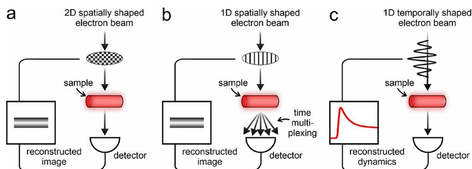
**Figure 1.** Single-pixel imaging with electrons. Schematic representation of different single-pixel schemes that are amenable to implementation in a transmission electron microscope for 2D spatial imaging (a), 1D spatial imaging (b), and 1D temporal reconstruction (c).
